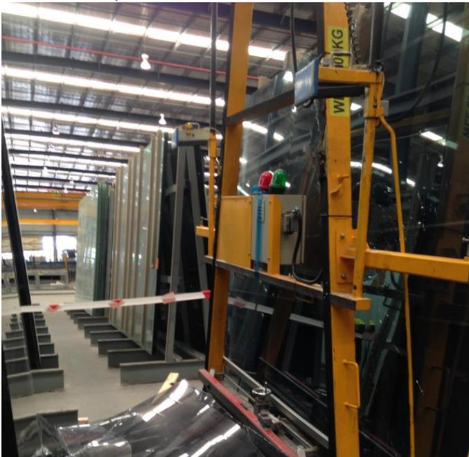
Even though the grab was fitted with the safe lift system, while lowering the pack onto the bearers the operator lost control of the pack. The pack did not have sufficient angle to keep it in position and it fell onto the operator.
